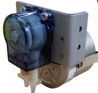
The 100 series, micro range of peristaltic pumps offer a low cost, compact & reliable means of dosing a wide range of liquids. They are available in various configurations of tubing type & size giving flow rates of between 0.016 & 0.26 ml/rev. The pump head is designed to be disposable but is assembled using a single screw enabling dis-assembly & re-assembly for tube changing if required.
