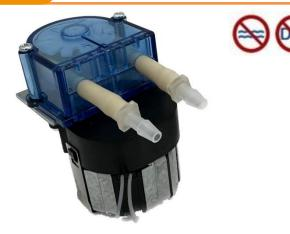
The 200 series, range of peristaltic pumps offer a low cost, compact & reliable means of dosing a wide range of liquids. They are available in various configurations of tubing type & size giving flow rates of between 0.1 & 1.32 ml/rev. The pump head is designed to be disposable but is assembled using a single screw enabling dis-assembly & re-assembly for tube changing if required. Important: These pumps are not suitable for use in wet or high humidity areas and
